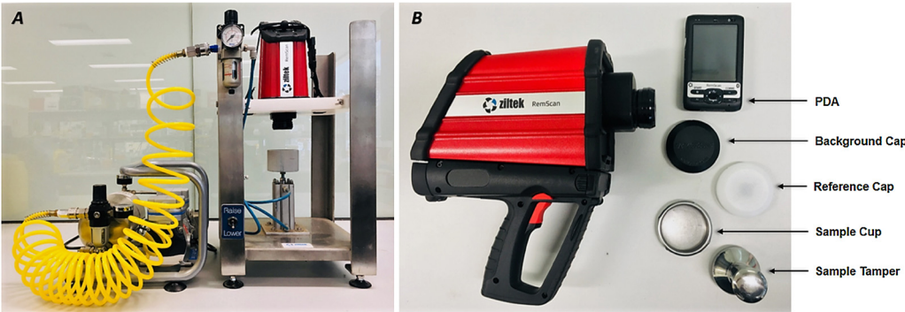
Fig. 1. (A) RemScan device installed on the Lab Station. (B) RemScan device and the related components.
